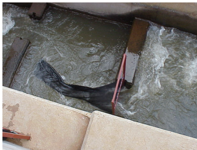
Plate 8.2: Placement of the long-bagged net in the notch of the baffle
