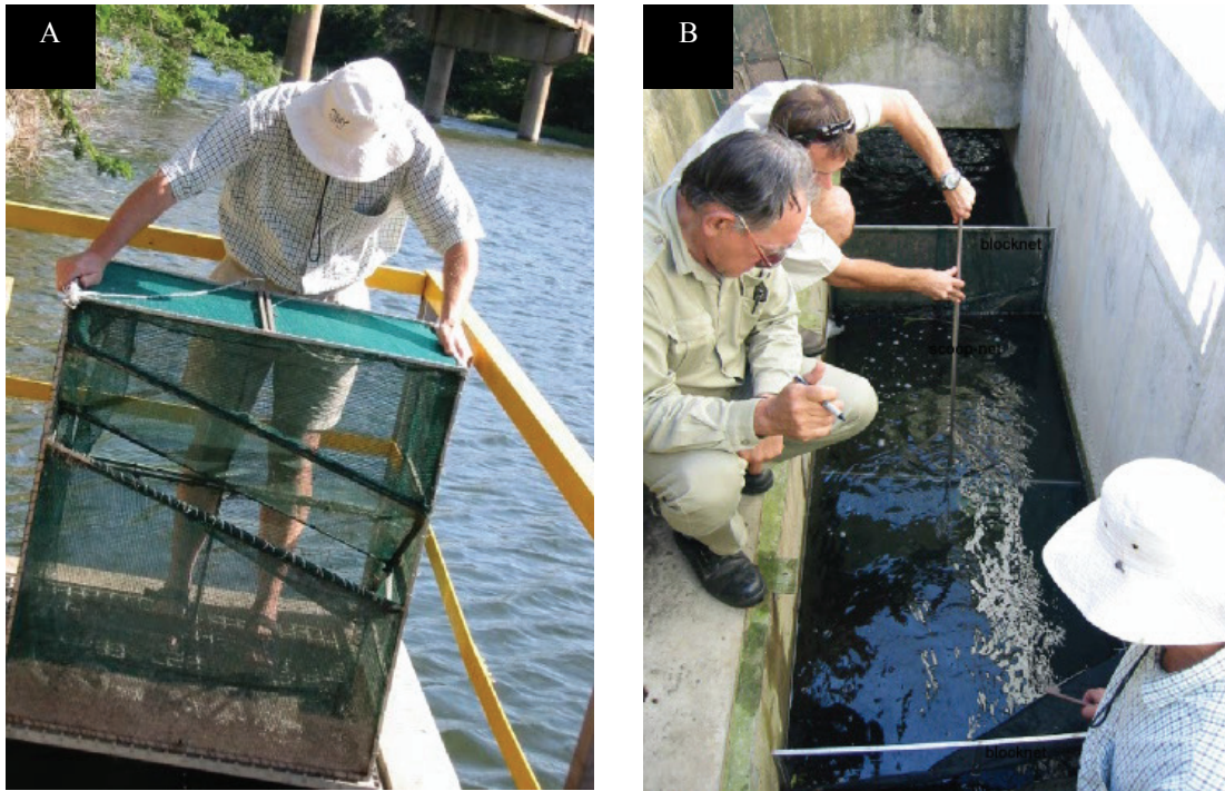
Plate 7.5: Funnel trap (A) and block nets (B) in pool 82 in fishway showing position of block nets and use of scoop net to clear trap.
