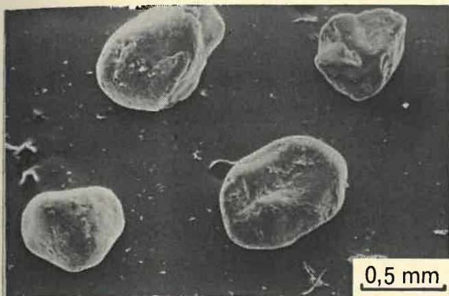
(a) A scanning electron photomicrograph of well rounded sand grains from the tidal inlet of the Swartkops estuary. This sand comes from the adjacent beach.
