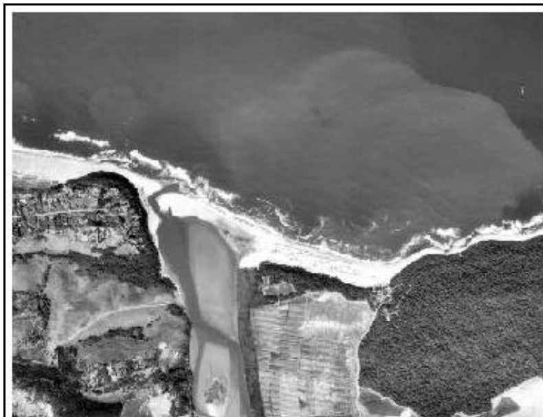
Fig 5.2 During low flow period fan is eroded, 2 August 1983
