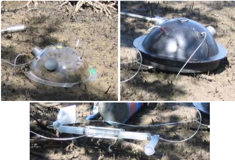
Figure 2. Microcosm apparatus used during September 2006, showing the light chamber, dark chamber and the closed circuit syringe system that was used to take samples.
