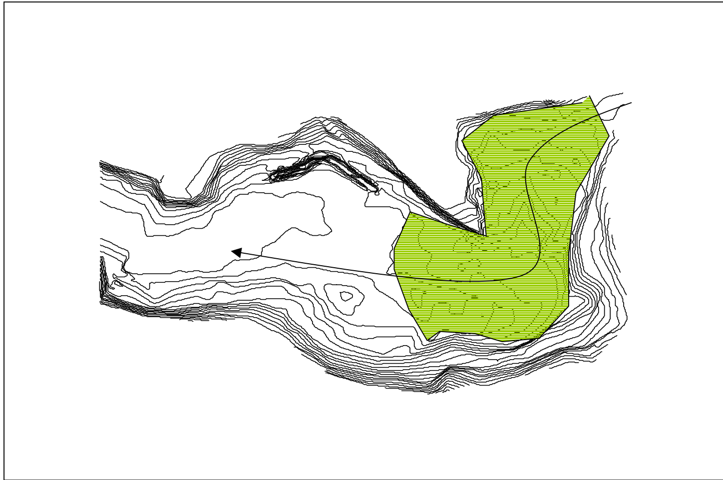
Figure E3: Topography of the Wadrif wetland (extent of wetland demarcated with green shaded area; arrow shows water flowpath)
