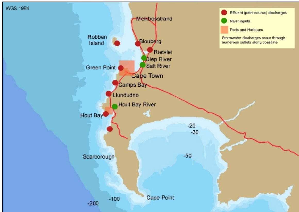
Figure 5.1: Potential marine pollution sources in the Cape Peninsula (western section)
