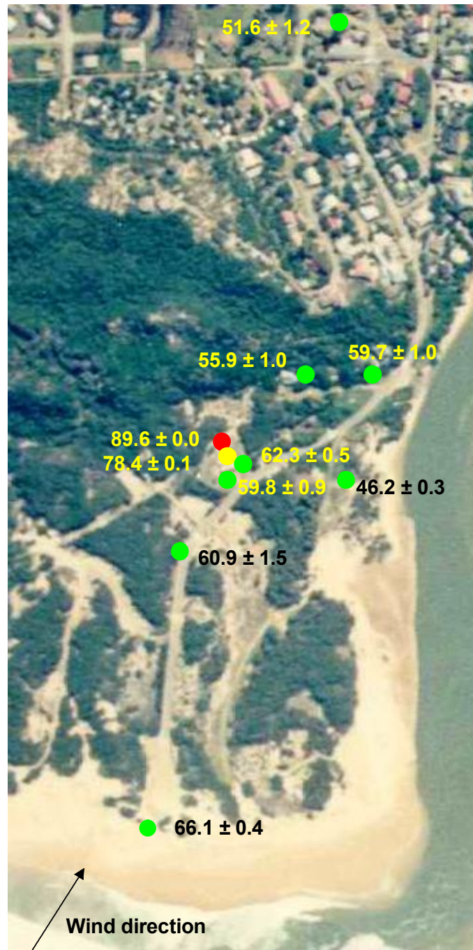
Figure 19. Sound pressure level measurements
