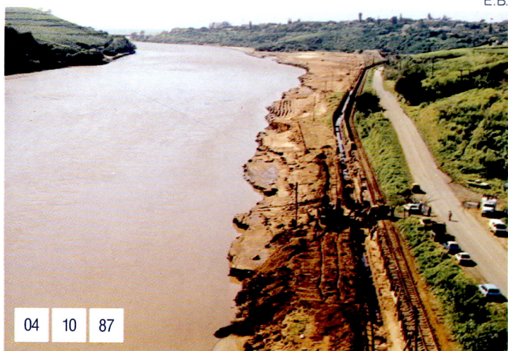
LOOKING DOWNSTREAM FROM THE FREEWAY BRIDGE: PRE & POST FLOOD. NB: VANISHED SUGAR CANE FIELDS & DAMAGE TO THE EFFLUENT CONDUIT
