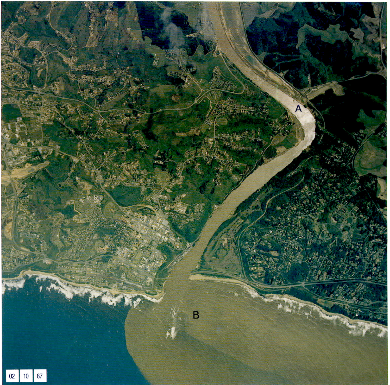
≈ 1:30000 A – LOW-LEVEL BRIDGE WASHED AWAY B – MASSIVE SILT PLUME
