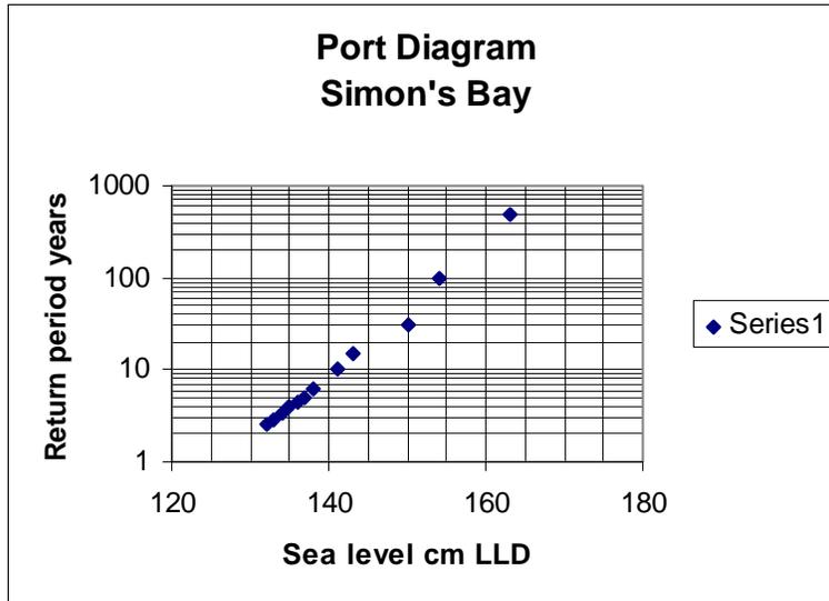
The observed annual maximum sea levels are used in the Simon's Bay Port Diagram for return periods up to 30 years, whilst the sea levels of LLD+154cm at a return period of 100 years and LLD+163cm for a return period of 500 years are extrapolations for illustration.
