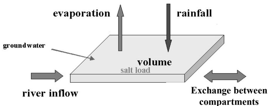
Figure 2: Schematic illustration of the hydrological balance of each compartment.
