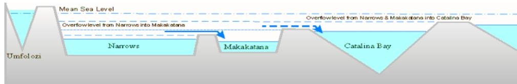
*Figure 3: Schematic illustration of the model. As water is inserted into the Narrows from the Umfolozi Link Canal, it will first spill over into Makakatana. The water level will then rise in both compartments until it spills over into the Catalina Bay. For the canal to be effective does not necessitate that the water level is raised to that of the combined Narrows-Makakatana basin – only that the salinity is diluted enough to remain below the 70-80 ppt.*
