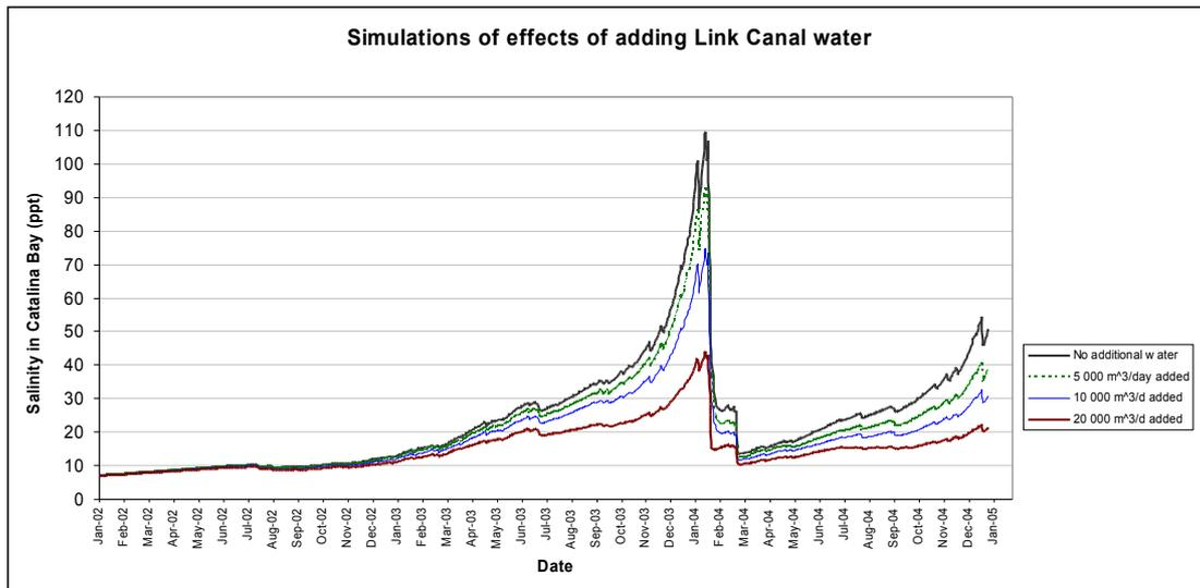
Figure 4: Simulations for the period Jan 2002 to Dec 2004 showing salinity levels without the addition of any water from the Umfolozi link Canal, and additions of 5000, 10 000 and 20 000 m<sup>3</sup>/day.
