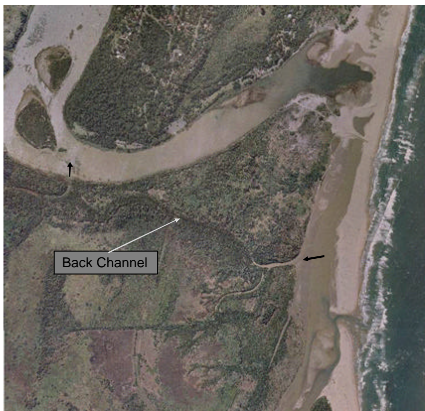
Figure 2: Ariel view of the Back Channel that will be opened to allow water from the Umfolozi Estuary to run into St Lucia Estuary once the Umfolozi mouth has been closed (Photo provided by R.Taylor).
