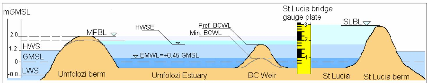
**Figure 3.15 Schematic showing key levels required for the functioning of the back-channel (not drawn to scale). BCWL is the Back-Channel Weir Level and MFBL/STBL are the Umfolozi and St Lucia Breaching Levels respectively.**
